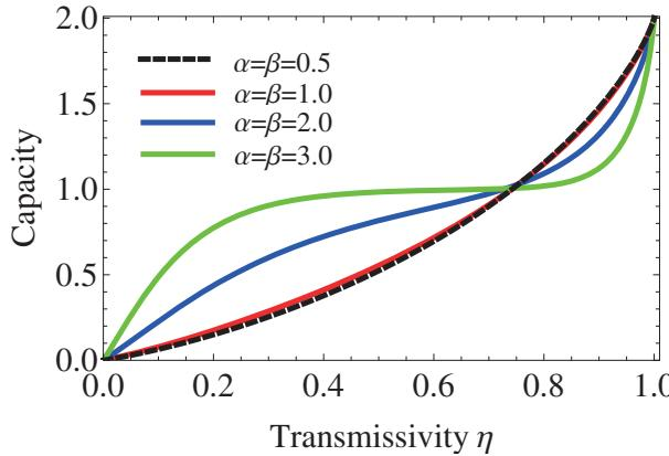
FIG. 2. Classical capacities assisted by quasi-Bell states with respect to the transmissivity  $\eta_A = \eta_B = \eta$  of the attenuated quantum channel. The black dashed line, the red solid line, the blue solid line, and the green solid line correspond to the cases that coherent amplitudes are  $\alpha = \beta = 0.5, 1.0, 2.0$ , and  $3.0$ , respectively.
