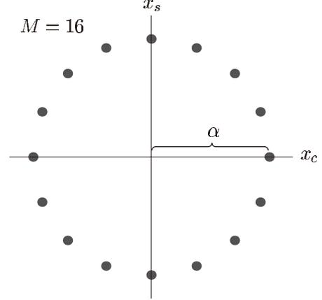
Fig. 2. Signal constellation of 16-PSK in  $(x_c, x_s)$ -plane ( $\alpha > 0$ )
