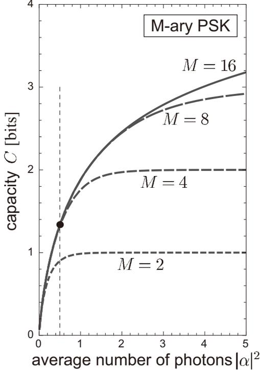
Fig. 3. Channel capacities of 2-, 4-, 8-, and 16-PSK signals.
