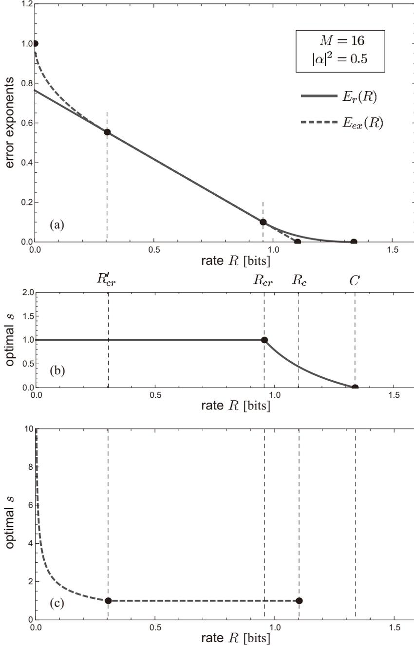
Fig. 4. (a) The random coding exponent, the expurgation exponent, and the zero-rate reliability function for 16-PSK coherent state signal; (b) The optimal  $s$  for the random coding exponent; (c) The optimal  $s$  for the expurgation exponent.
