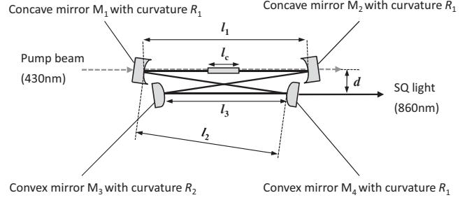
Fig. 3. Optical configuration of newly designed optical parametric oscillator.
