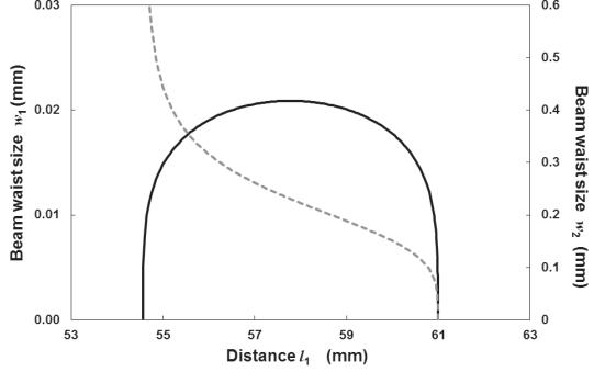
Fig. 2. Calculation results of  $w_1$  and  $w_2$  based on the conventional bow-tie cavity. Solid line and dashed line are representing the  $w_1$  and the  $w_2$  respectively.
