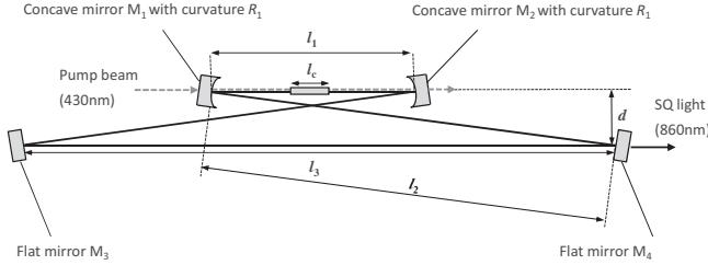
Fig. 1. Optical configuration of conventional optical parametric oscillator.
