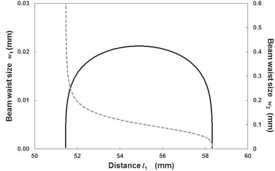
Fig. 4. Calculation results of  $w_1$  and  $w_2$  based on newly designed bow-tie cavity. Solid line and dashed line are representing the  $w_1$  and the  $w_2$  respectively.
