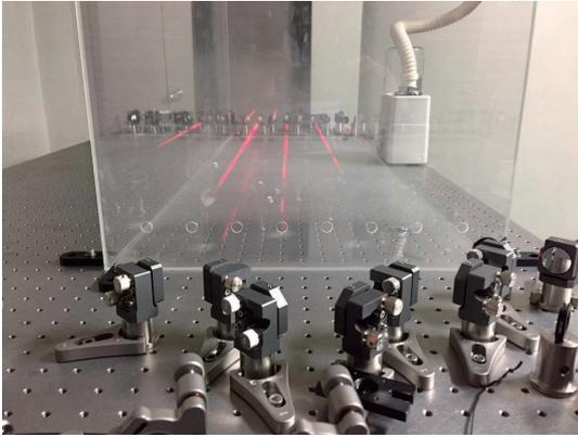
Fig. 2. Photograph of the fog chamber installed in the optical path of the signal beam.
