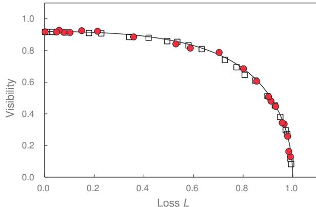
Fig. 3. Results of visibility measurement and calculation results. Open squares are experimental results using a neutral density (ND) filter instead of the fog chamber. Solid circles are experimental results with the signal beam propagating through 10 m length of a foggy atmosphere. Solid curve is calculation results assuming only the optical energy loss  $L$ .
