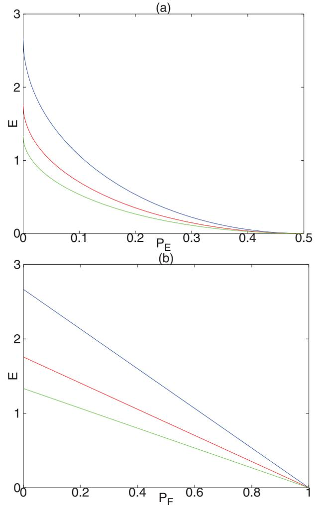
FIG. 1. (Color online) Optimal tradeoff between the energy  $E$  and the probability of error  $P_E$  (probability of failure  $P_F$ ) in the ambiguous (a) and unambiguous (b) discrimination of  $I$  and  $U = \exp(i(\delta a_1^\dagger a_1 - \delta a_2^\dagger a_2))$ , for  $\delta = \pi/6$  (upper line),  $\delta = \pi/4$  (middle line), and  $\delta = \pi/3$  (lower line), as given by Eq. (11).
