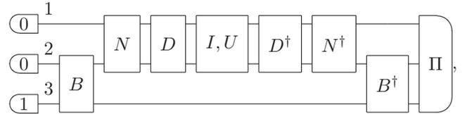
where  $N$  is a 50/50 beamsplitter,  $I, U$  is the unknown beamsplitter, and  $D$  is the beamsplitter diagonalizing  $U$ . The POVM  $\Pi$  is different for ambiguous and unambiguous quantum reading. It is easy to verify that the composition of beamsplitters  $DN$  reduces to a phase shifter on mode 2, namely
